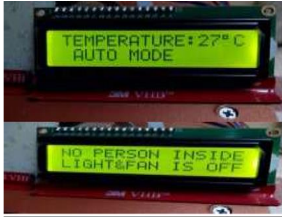
Fig.5: LCD displaying Automatic Mode
